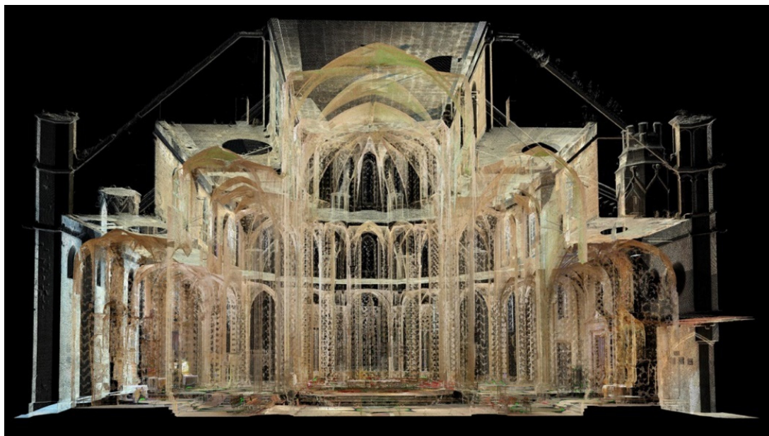
Figure 7. An image resulting from the terrestrial laser scanner (TLS) survey of the apse of the Tortosa Cathedral.
