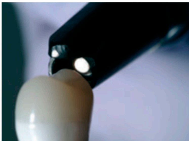
Figure 3. The periometer and its probe with percussion rod. Probe pulled back to show percussion rod—that was used in the study [64].
