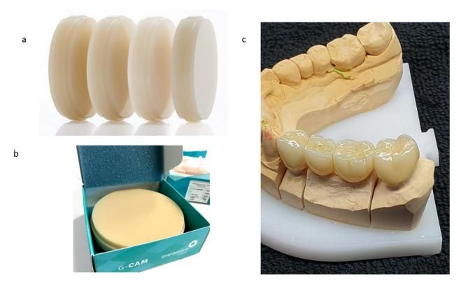
**Figure 1.** (a). Color range of PMMA–graphene offered by the manufacturer. (b) Samples studied as G-PMMA. (c) Dental restoration with G-PMMA with excellent esthetic results.
