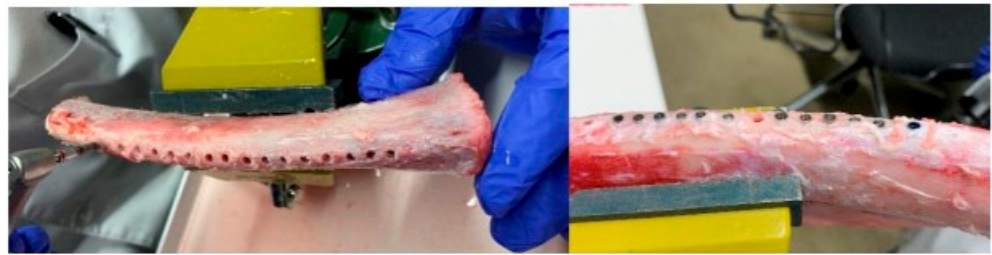
Figure 2. Bone level dental implant inserted in the fresh cow ribs.
