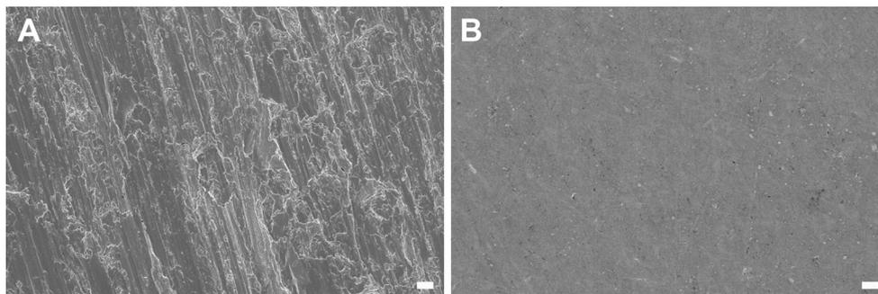
**Fig. 3** Scanning electron microscope images. **a** Trimmed Ta samples before polishing. **b** Smooth Ta samples after polishing. Surface activation treatments rendered similar micrographs as observed for smooth control samples (**b**). Scale bar = 2 μm
