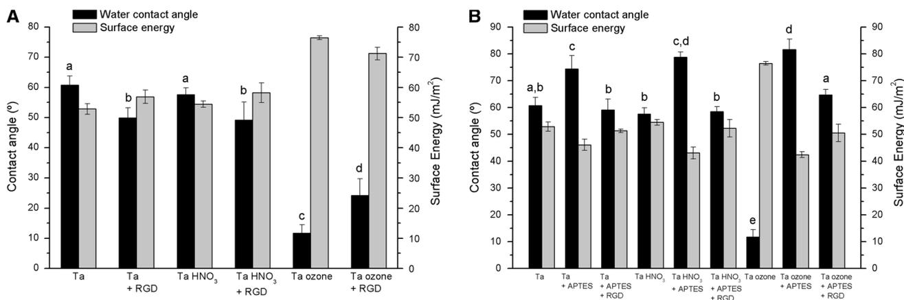
**Fig. 4** Water contact angle measurements and surface energy calculations. **a** Activation of Ta samples (Ta) by passivation (Ta HNO<sub>3</sub>) or UV/ozone treatment (Ta ozone), and physical adsorption of RGD peptide (+RGD). **b** Activation of Ta samples (Ta) by
