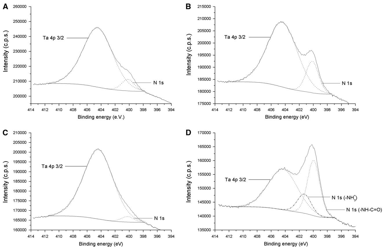
**Fig. 5** Curve-fitting deconvolution of high resolution XPS spectra (Ta 4p 3/2 and N 1s signals). **a** Control Ta samples (Ta). **b** Physical adsorption of RGD peptide on control surfaces (Ta + RGD). **c** Physical adsorption of RGD peptide on UV/ozone-treated surfaces
