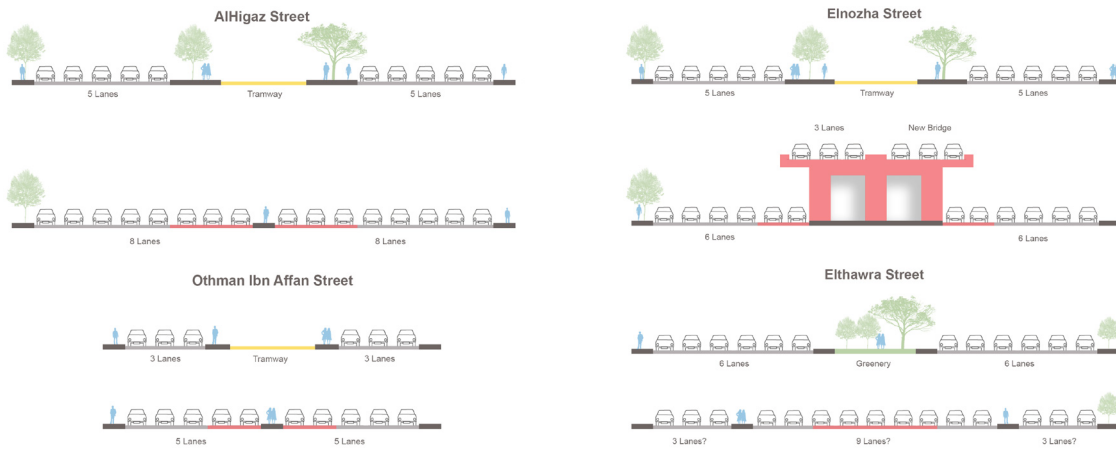
Figure 18 Before/after street sections of some roads that have been affected by the urban changes. The author approximates road capacities according to multiple Google Earth and Google Maps satellite images of the streets.
