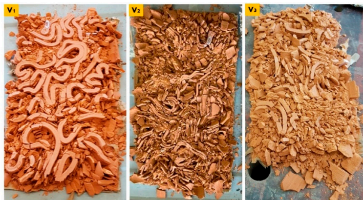
Figure 12. Exhibits comparison between the cumulus of three linear model bricks, V1, V2, and V3, post-collapsing as a result of the compression test. It can be observed that the V1 exhibited the highest resistance since it maintained many of its parts, followed by the V3. At the same time, the V2 recorded the least compression resistance as it was the most affected, as shown in the figure.
