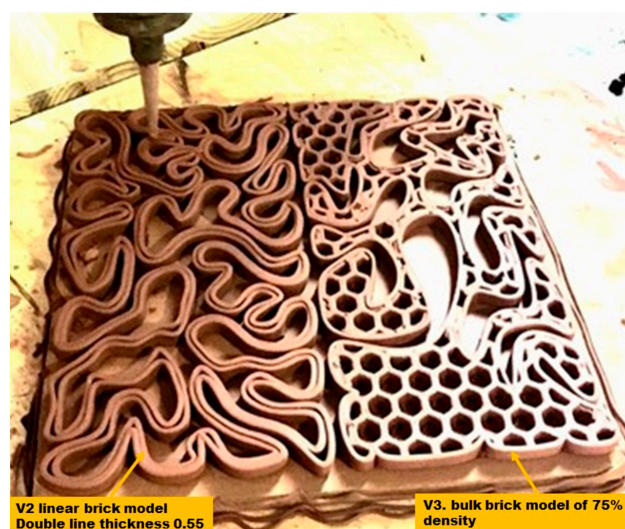
Figure 2. The 3D printing process of the 3D-printed biodigital clay bricks exhibiting the differentiation in printing settings between the linear model (V2) of double line each of 0.55 cm thickness and a bulk model (V3) with honeycomb infill. 3D printing managed by La Maquina by Noumena. (Photo by authors).
