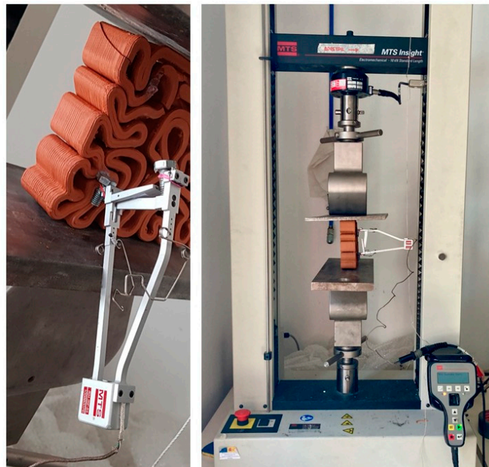
Figure 3. Showing the device used to apply the elasticity test of the 3DPBDCB, using the MTS Insight 10 kN electromechanical press. At the facilities of the CATMech-Litem research group (ESEIAAT School, UPC). (By authors).
