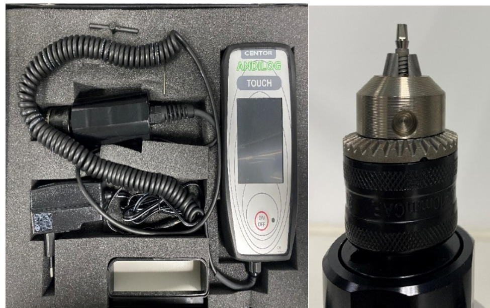
Figure 4. Digital Torque Gauge with the chuck to hold the samples.
