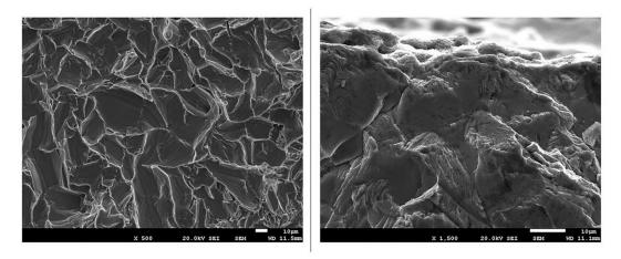
**Figure 7.** SEM images at a magnification of ×500 and ×1500 showing the striations from the fractography.
