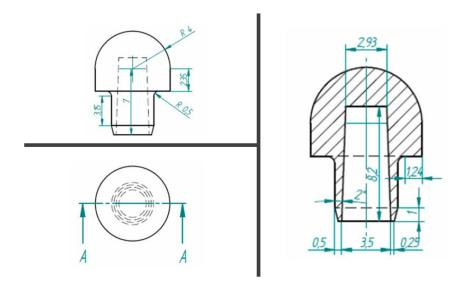
Figure 2. Spherical member of the load application design details.
