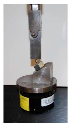
Figure 3. Load cell over the sample in the testing machine.
