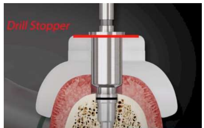
Figures 11 (left) and 12 (right): Illustration of the contact between drill and surgical guide (Images provided by Osstem)
