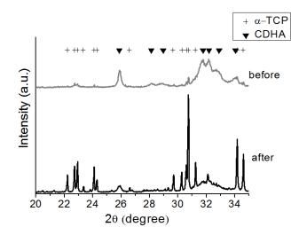
**Figure 1.** XRD patterns of the CPC powders, showing initial alpha-TCP phase that transformed completely to calcium-deficient hydroxyapatite (CDHA) after immersion for 7 days.
