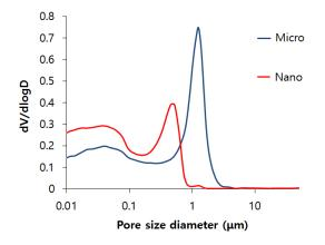
**Figure 3.** Characterization of pore size distribution of hardened CPC samples, showing nano-sized pores in the nano-CPC and micro-sized pores in the micro-CPC.
