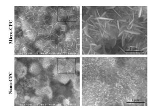
Figure 2. SEM images of micro- and nano-CPC at different magnifications.
