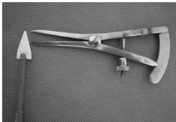
Figure 1 Polyvinyl alcohol sponge and compass used to measure 6 and 8 mm from the tip, to create TS6 and TS8, respectively.
