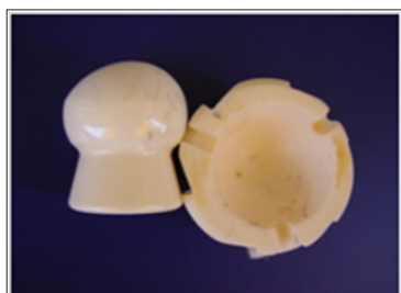
Figure 1: Clinical case 1: Macroscopic wear of the retrieved CoC THR first generation retrieved liner.
