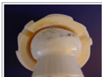
Figure 2: Clinical case 1: Macroscopic wear of the retrieved CoC THR first generation retrieved femoral head.
